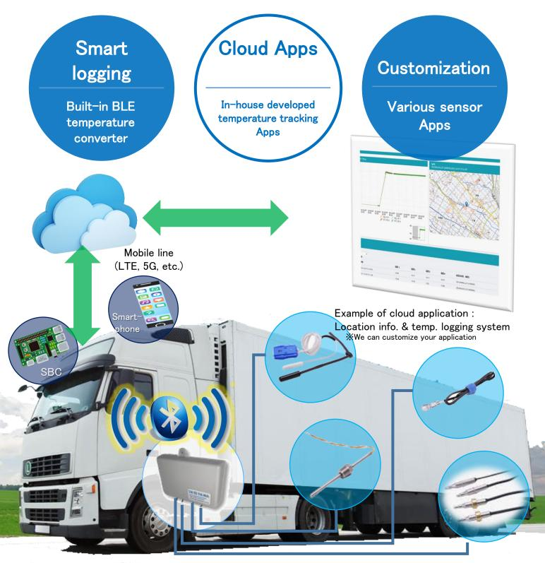
Maximum analog signal length: 20 m (up to 4 temp. sensor per unit)
