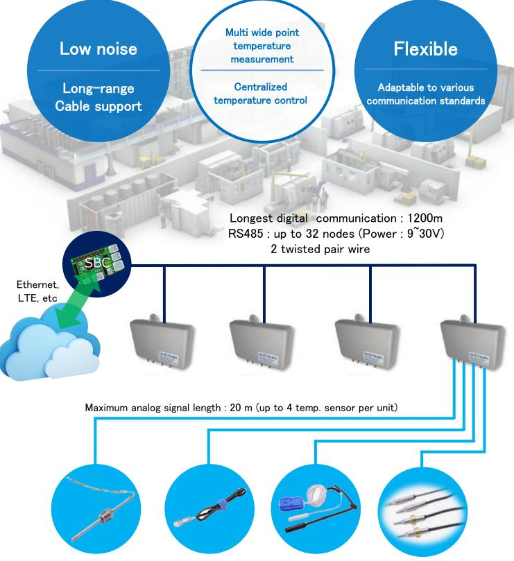
Data acquisition possible with up to 128 temperature sensors (=32 nodes x 4 sensors)
